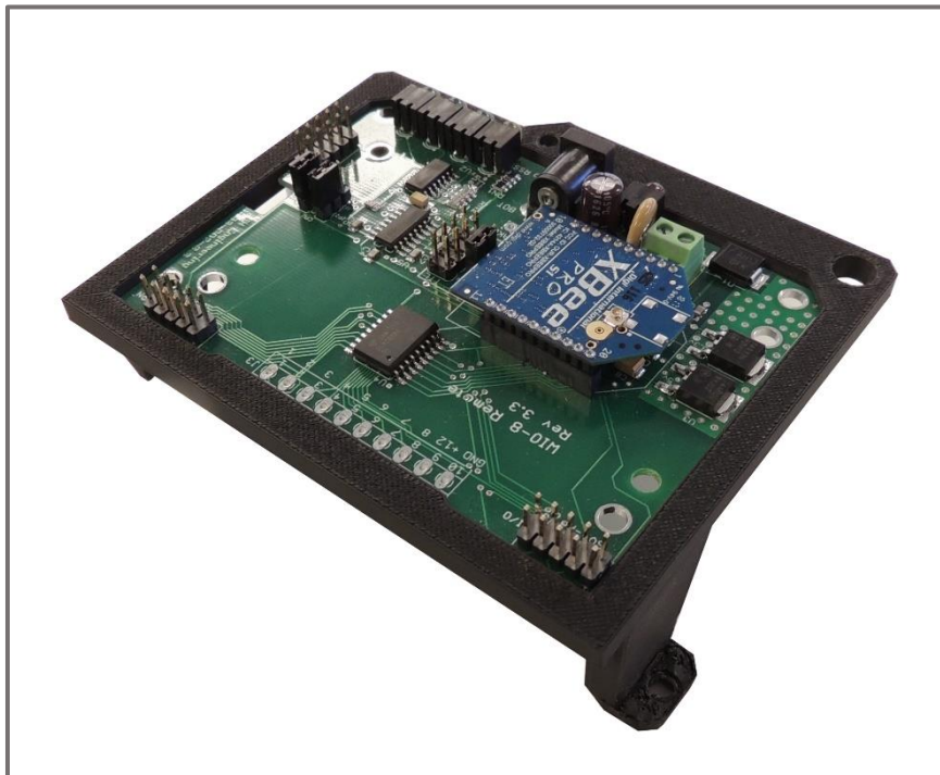
Fig. 8 Mounting bracket with GHE remote board and Wi-Fi module installed.
