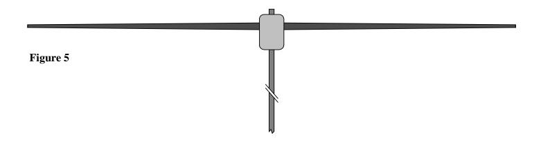
When the control cable and coax have been connected you can tape the two cables together for the run to your shack. Be sure to leave a proper loop at the mast to allow for the turning of the rotor.
