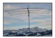
**The DB18E Yagi** is identical in every way to the DB18, with one exception—the DB18E utilizes three active loop elements on 30m, which provides outstanding performance on the 30m band. The DB18E has two active elements on 40m and three active elements on 30m-6m. The picture to the left is the snowy QTH of HB9CVE.
