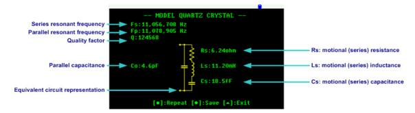
The process starts by searching for the series and parallel resonant frequencies. The start scan frequency is taken from the specified frequency value. The scan range is +1 MHz up and -1 MHz down from this value.
