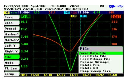
After selecting the *«Save Data File»* submenu option, enter the file name. By default, the file name has the format *"sark\_\_xx.csv"* (or *"sark\_\_xx.tdr"* for Cable Test mode), where xx is an automatically assigned number. To change the file name, use Navigator B to change the character value and Navigator A to change the character position highlighted in inverse video. Press the Select **[**] button to validate the selection. Press any other button to cancel the operation.
