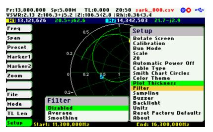
The *«Average»* filter minimizes the noise but at the expense of reducing the measurement speed. Four samples are taken for each measurement frequency and an average from these samples is calculated.
