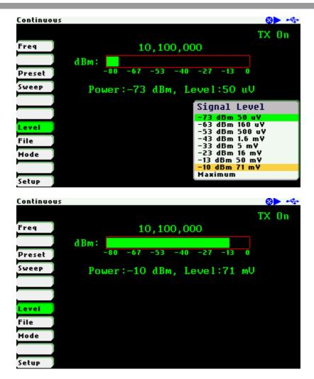
The signal generator outputs continuously unless it is paused by pressing the Run/Hold [>||] button. In the Hold state the level graph and power level indicators change to red. Signal generation can be resumed at any time by pressing the Run/Hold [>||] button again.
