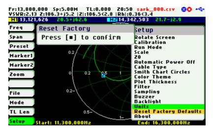
The internal disk drive can be optionally formatted. Press the Select [] button to format the disk or any other button if only a reset to factory defaults is required.
