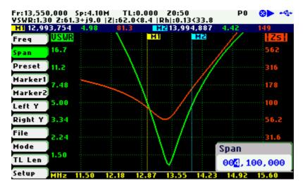
(ii) Use Navigator A to highlight «Span» in the main menu on the left side of the display. Then use Navigator B to change the span. The span will change according to the current span frequency multiplier. The span frequency multiplier can be changed from the popup dialog, see
