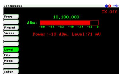
In frequency sweep mode the signal frequency will sweep between two user-defined frequencies. To change the sweep parameters, use Navigator A to highlight **«Sweep»** in the main menu and press the Select [] button to validate the different sweep parameters.
