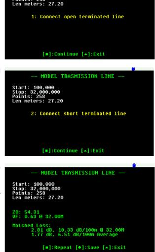
**Note:** Try to keep the electrical length of the line exactly the same between the open and short termination conditions. Ideally you would terminate the line with the same standard loads that were used to do the Open Short Load (OSL) calibration.
