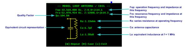
The internal procedure performed by the analyzer is as follows: the analyzer measures the impedance at 1 MHz and at the desired operating frequency (e.g. 13.56 MHz). Then it searches for the antenna's self-resonant frequency and measures the impedance at that point. The following parameters are extracted from these measurements:
