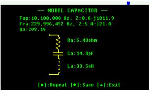
The figure below describes the measured parameters:
