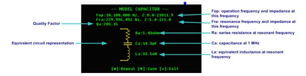
The internal procedure performed by the analyzer is as follows: the analyzer measures the impedance at 1 MHz and at the desired operating frequency. Then it searches for the self-resonant frequency and measures the impedance at this point. The following parameters are extracted from these measurements:
