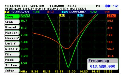
(ii) Use Navigator A to highlight **«Freq»** in the main menu on the left side of the display. Then use Navigator B to change the frequency. The frequency will change according to the current frequency multiplier. The frequency multiplier can be changed from the popup dialog, see (i) above.
