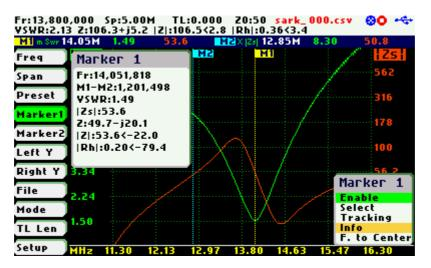
The *«F. to Center»* menu option can be used to set the centre frequency at the marker's frequency value.
