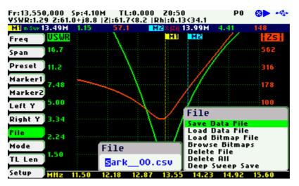
The *«Save Data File»* option can be also selected by pressing Navigator A when *«File»* is highlighted.
