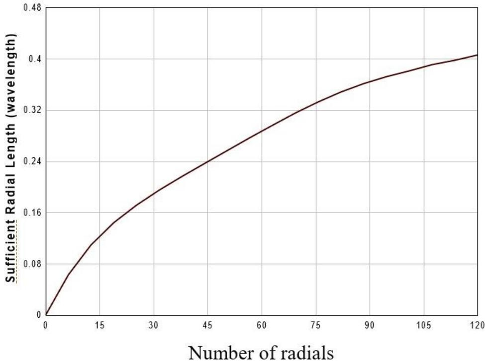
If you cannot lay the radials out in a symmetrical radial pattern, don't worry too much - it will distort your omni-directional pattern slightly but won't reduce the efficiency by much. Lay the radials out in the best manner possible given your situation.
