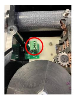
Align holes in copper beryllium (Cu-Be) tape to the screws that hold the EHU contact brush in place (circled in red).
