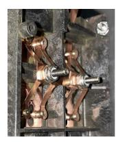
• If you are completing this process on a driven EHU (internal balun) you will need to de-solder the brushes and re-solder the new ones onto the internal balun ring lugs. Use an alligator clip fixture or some other way of holding the ring lug while de-soldering the brush.
