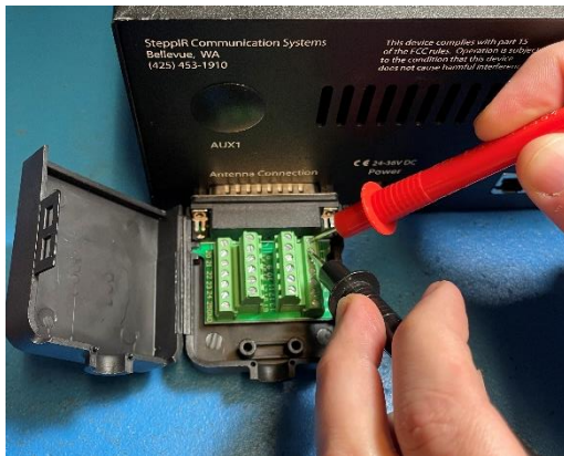
Figure 5: Spare DB25 field splice voltage measurements
