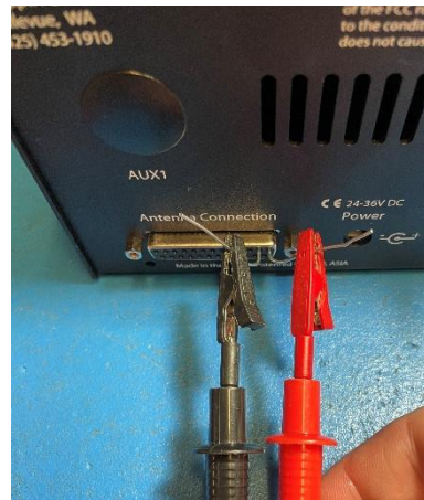
Figure 6: Direct voltage measurements with clips
