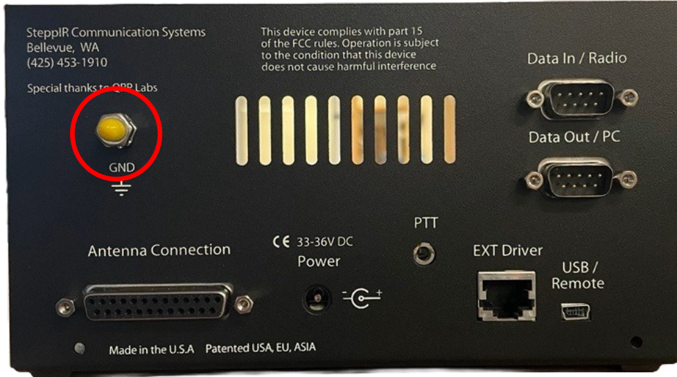
Figure 8.05: Lug location for OptimizIR 2.0 (stainless steel chassis)
