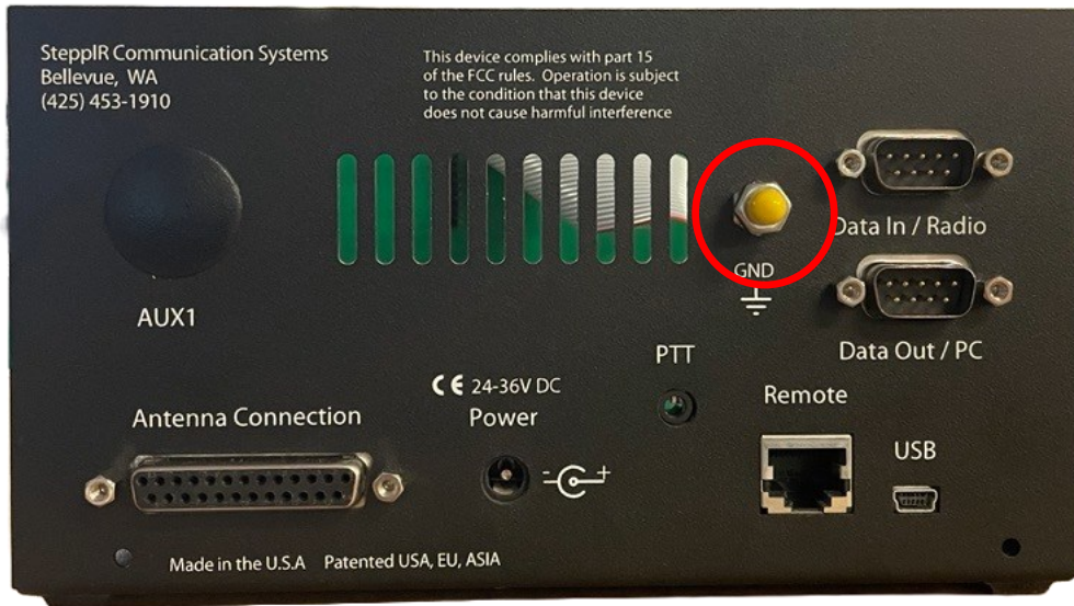
Figure 8.04: Lug location for SDA100, OptimizIR, and OptimizIR 2.0 (early models)
