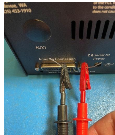
Figure 6: Direct voltage measurements with clips
