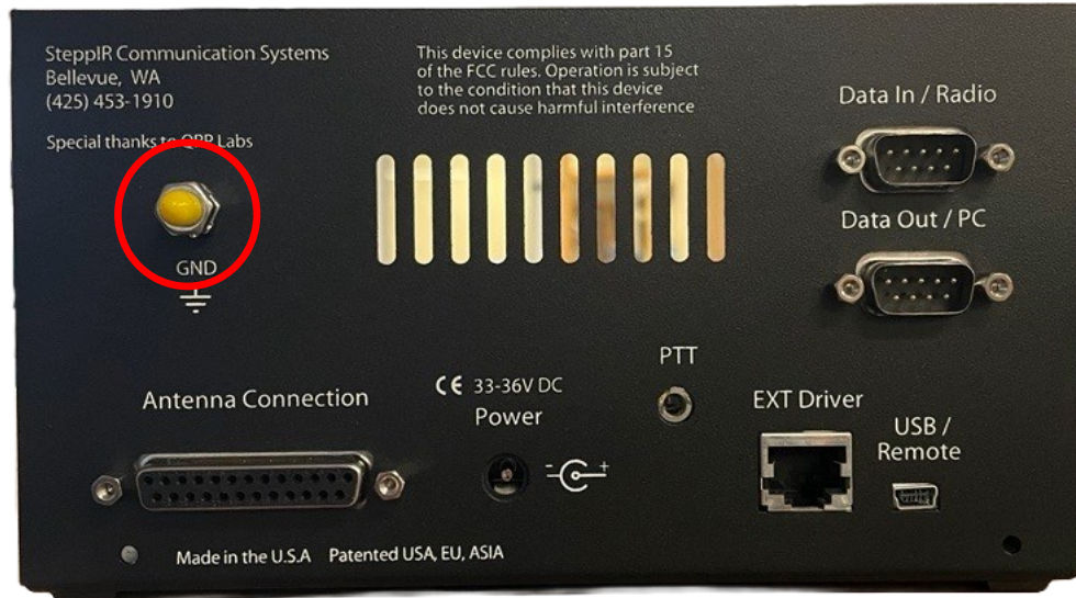
Figure 8.05: Lug location for OptimizIR 2.0 (stainless steel chassis)
