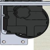
Our new reinforced DB mounting plate assembly for the element housing unit (EHU) is significantly stronger. This design redirects stress from the forces on the fiberglass poles away from the EHU and directly to the boom, greatly reducing the potential for damage in high winds or ice loading!
