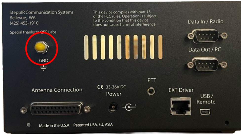
Figure 6.06: Lug location for OptimizIR 2.0 (stainless steel chassis)
